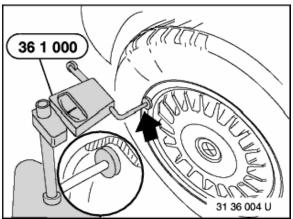
Check radial runout of rim with special tool 36 1 000 (measuring fixture),
