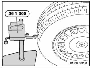
Check wheel for radial runout with special tool 36 1 000 (measuring fixture),
